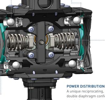
A unique reciprocating, spring driven, double diaphragm configuration retains constant pressure, regardless the load. Motor amperage is actually reduced as back pressure increases. No internal bypass. Pump automatically goes neutral when end-of-hose valve is shut off.
