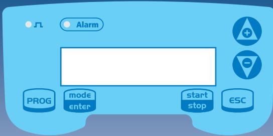
Digital interface version; Timer function; Ppm proportional dosing; Statistics; Password; Input On-Off (remote control). Constant flow rate manually adjustable, proportional flow rate according to an external analog (4-20 mA) or digital signal (water meter)
